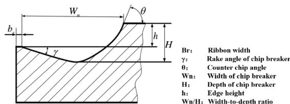
Figure 3: Basic structure of chip breaker
