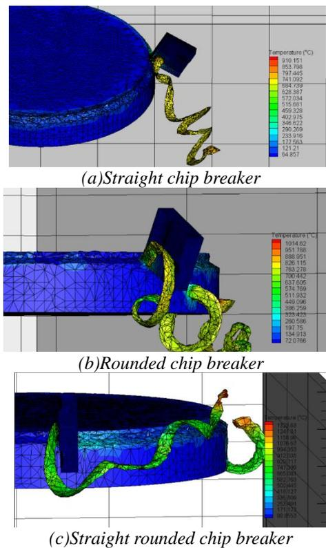
*Figure 4: Cutting patterns with different chip breakers*
