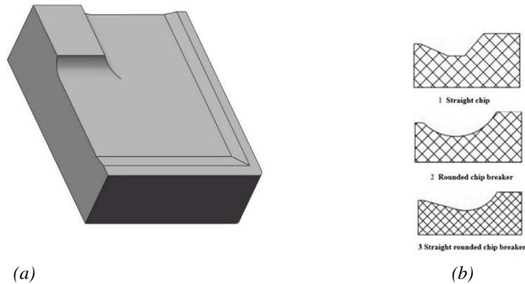
*Figure 1: 3D model of the cutting part of the tool with different chip breakers*
