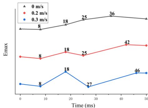
Figure 4: Variation curve of the maximum field strength  $E_{max}$  inside the bubble at different flow rates in the horizontal oil channel
