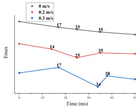
Figure 6: Variation curve of the maximum field strength  $E_{max}$  inside the bubble at different flow rates in the vertical oil channel
