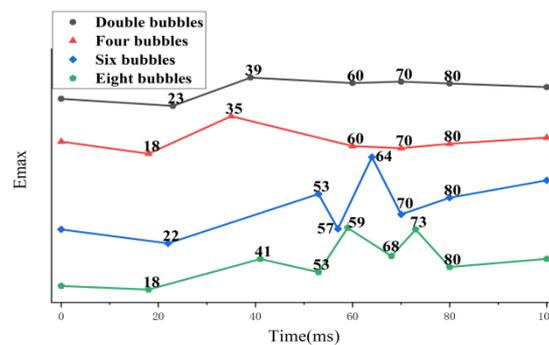
Figure 8: Variation of the maximum field strength  $E_{max}$  inside the bubble for different numbers of bubbles in the dual oil channel model
