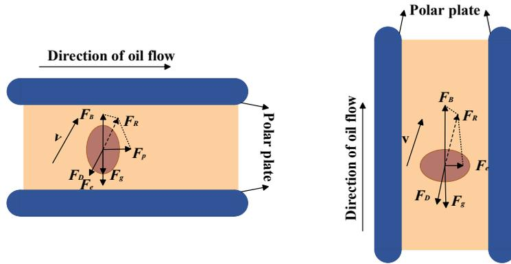
(a) Force analysis of air bubbles in horizontal oil channels (b) Force analysis of air bubbles in vertical oil channels
