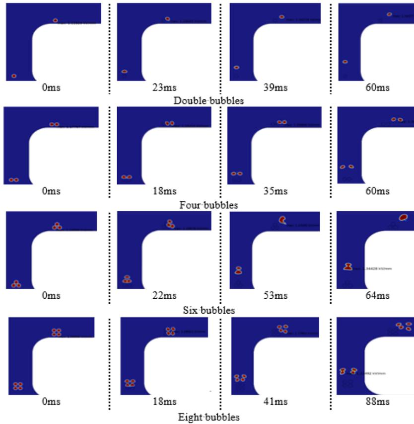
Figure 7: Bubble motion characteristics for different numbers of bubbles in a dual oil channel model
