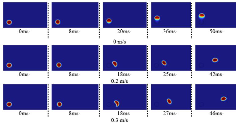
Figure 3: Bubble movement characteristics in horizontal oil channels at different oil flow rates
