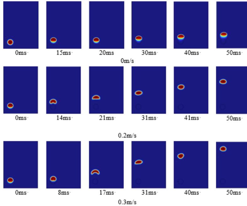
Figure 5: Bubble movement characteristics at different oil flow rates in vertical oil channels
