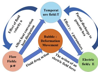
Figure 1: Coupled electric-temperature-flow field model for insulating oils containing air bubbles
