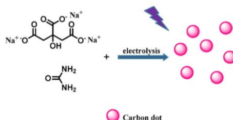
Figure.2 The Formation of the CDs by Electrochemical Approach
