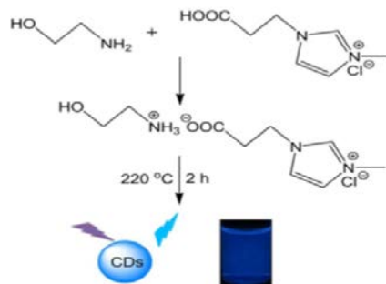
Figure.4 Schematic Representation of Synthesis Procedures of CDs.
