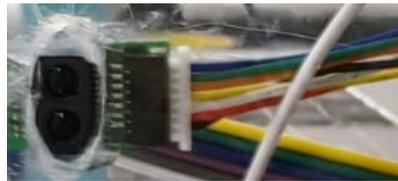
Figure 4: Infrared ranging module
