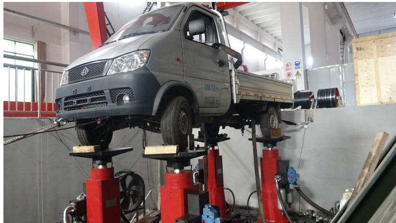
Figure.5 Missile transportation sweep frequency test.
