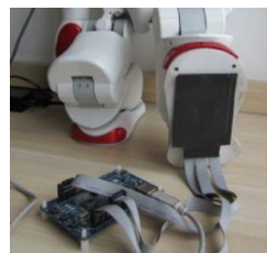
Figure 8: Sensor adhered to the foot of NAO
