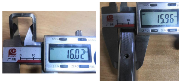
Figure 11: Measured dimensions of the matching surface of lock pin sleeve and lock pin
