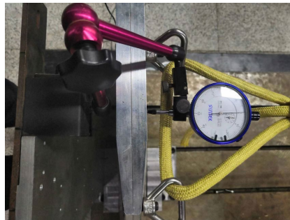
Figure 10: Displacement measuring tool for the rudder tip chord
