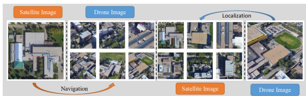
Figure 1: Cross-view geo-localization and navigation based on satellite and UAV images.
