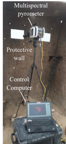
Figure 2 The experimental setup for measuring a TNT explosive fireball
