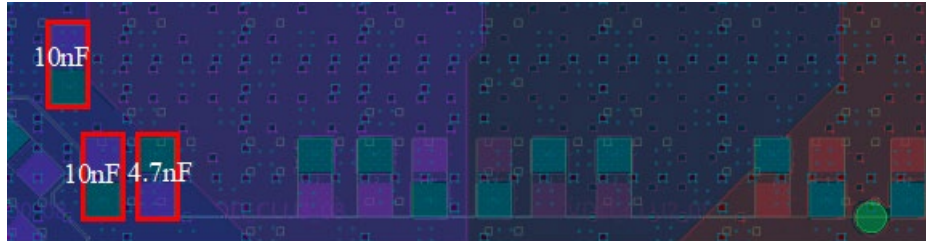
Figure 11: Decoupling capacitors of VDD_CLU0.
