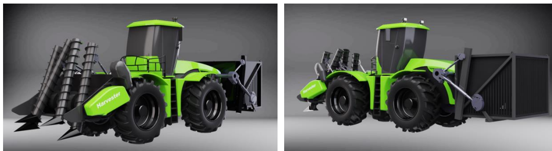
Figure 3: Final design scheme of sugarcane harvester
