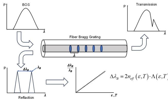
*Figure 1: Basic working principle diagram of FBG sensors*
