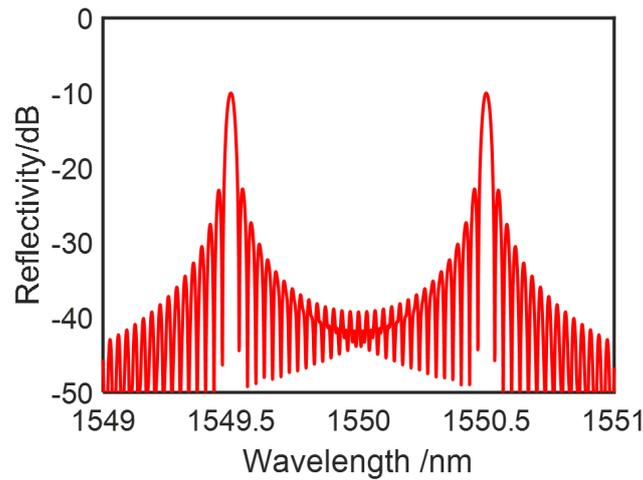
Figure 5: The reflection spectrum of two cascaded FBG
