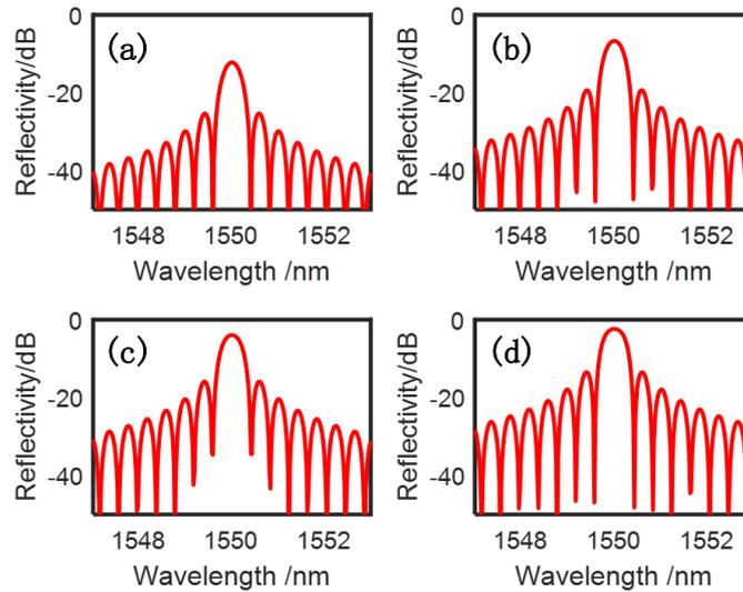
Figure 3: FBG reflection spectra with different  $\kappa$
