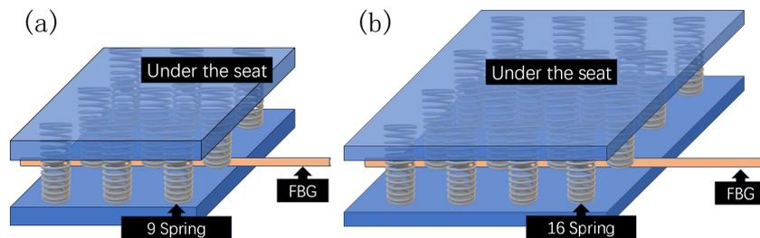
Figure 8: Schematic diagram of a single-seat fiber Bragg grating spring package
