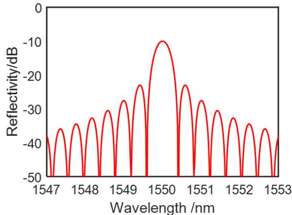
Figure 2: The reflection spectrum of a single FBG
