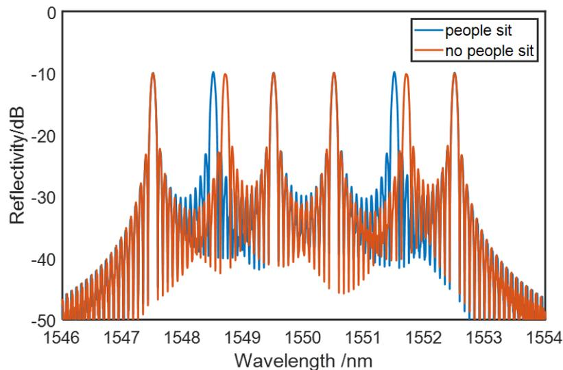
Figure 9: The reflection spectrum of six cascaded FBG when people sit down or not
