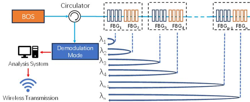
Figure 7: The diagram of a real-time monitoring system for student sitting conditions based on a weak reflective fiber grating array
