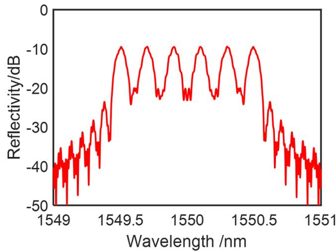
Figure 6: The reflection spectrum of six cascaded FBG
