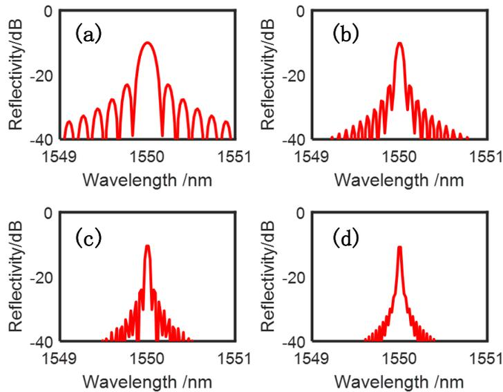
Figure 4: The reflection spectrum of FBG at different grating lengths L
