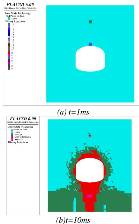
Figure 7: Cloud Map of the Plastic Zone of the Modelled Dielectric Cell
