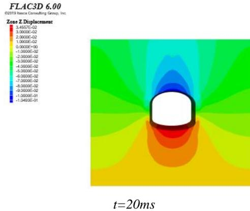
Figure 6: Vertical Displacement Distribution of the Model
