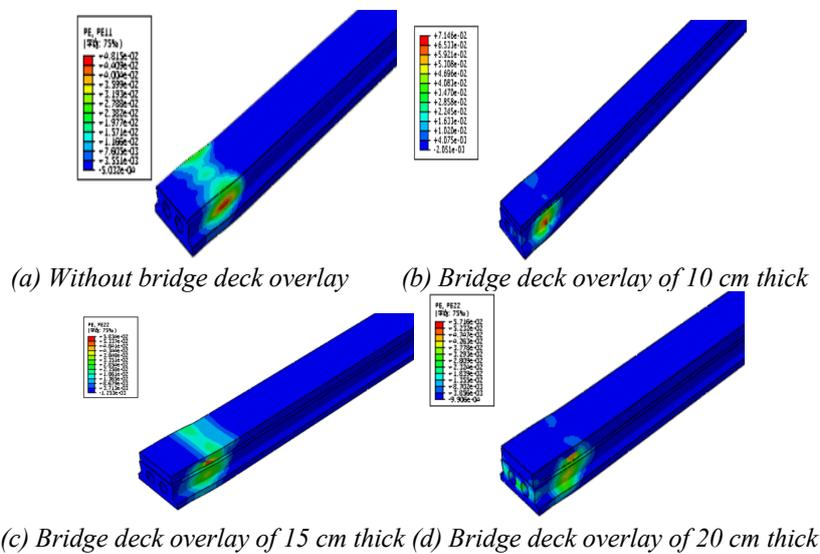
Figure 6: Cloud pictures for strain of the voided slab
