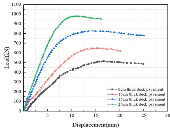
Figure 7: Load-displacement curves in the finite element simulation
