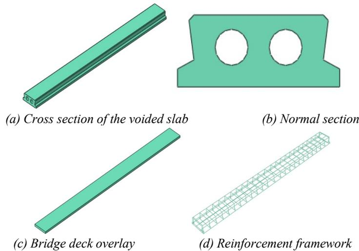
Figure 2: Main components of the model
