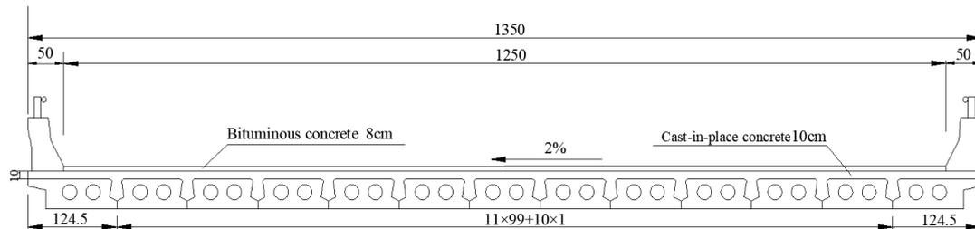
Figure 1: Cross section of the voided slab bridge (unit: m)
