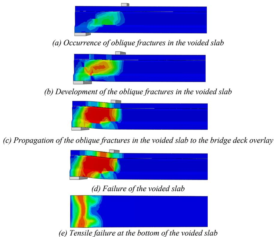
Figure 5: Failure modes of the voided slab obtained in the finite element simulation
