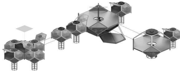
Figure 8: Rules for aggregation of modular residential space
