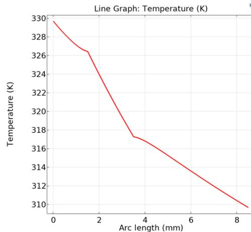
Figure 9: Temperature curve of XLPE layer in the presence of bubble defects
