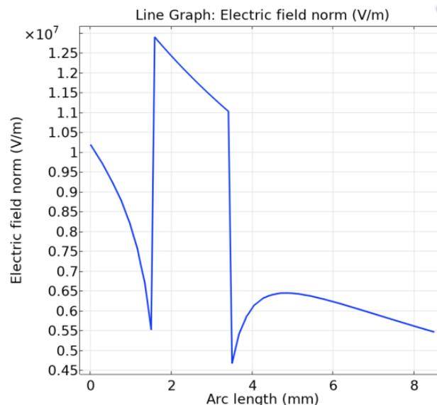
Figure 8: Field intensity curve of the XLPE layer in the presence of bubble defects
