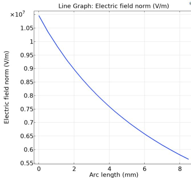
Figure 5: Electric field intensity curve of the XLP Elayer
