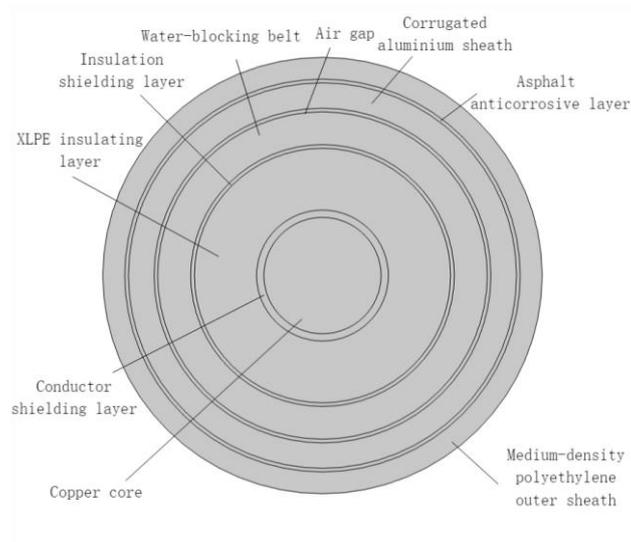
Figure 1: A crosslinked polyethylene cross-section model
