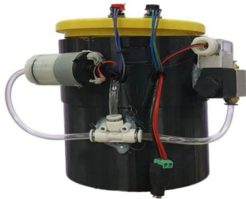
Figure 4: Exterior Structure of the First Generation Prototype
