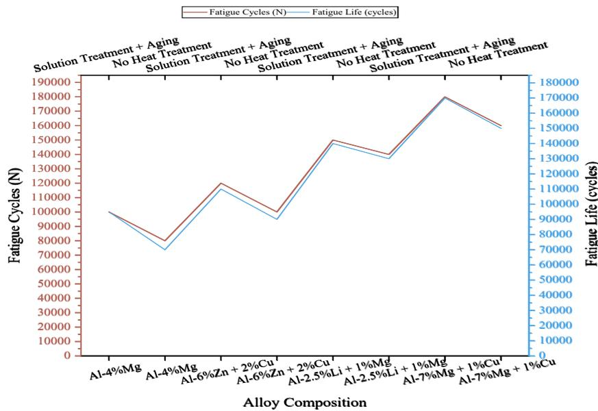
Figure 4. Fatigue life of high cycle fatigue test
