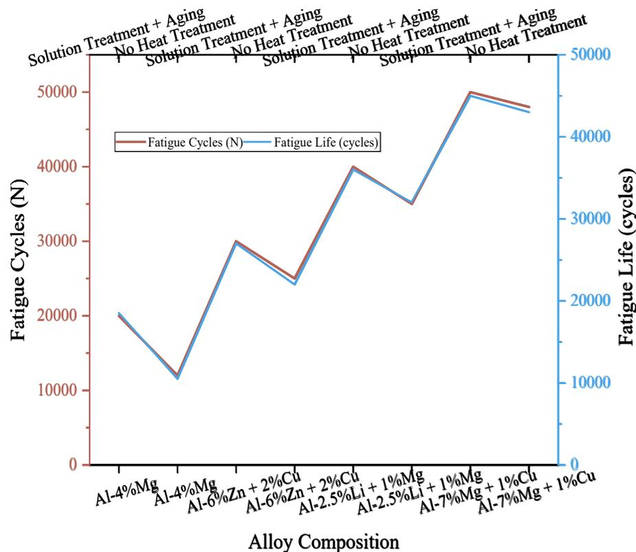
Figure 2. Fatigue life of low cycle fatigue test
